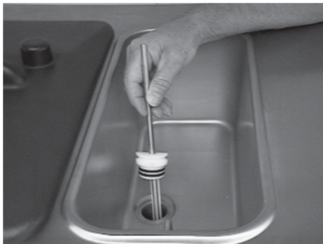
Figure 17. Removing Mix Inlet Regulator
